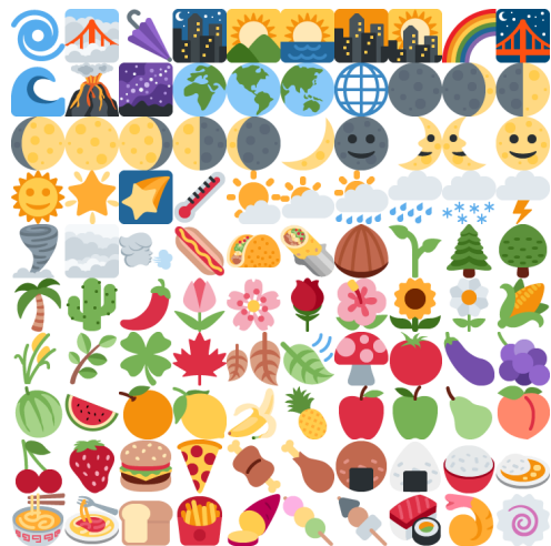
Figure 1. A 100-tile atlas (10x10 grid of 72x72px tiles, 720x720px). Encoded with identical encoder settings both ways (distinct from Table 1’s matched-quality protocol), the 100 tiles cost 147,361 bytes as separate JPEG files and 112,059 bytes as this single JPEG (24% less), while 100 HTTP requests become one. Each tile is displayed with CSS background-position.
